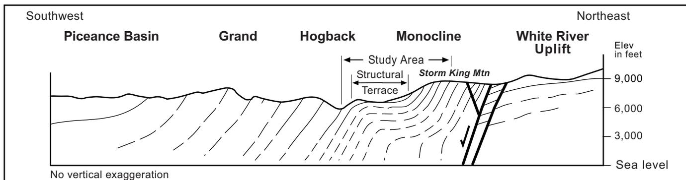
**Figure 7. Schematic structural cross section from the Piceance Basin on the southwest to the White River Uplift on the northeast, showing the relative position of the structural terrace within the Grand Hogback Monocline and the location of the study area. Individual formations are not depicted; only the generalized attitudes of bedding and major faults are shown. Cross section based upon Bryant and others, 1998.**
