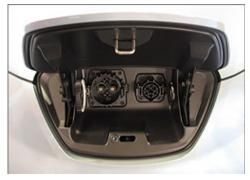
**Figure 1:** The standard receptacle (right) can receive charge from level 1 or level 2 equipment. The DC fast charge receptacle (left) uses a different type of connector. Photo courtesy of National Renewable Energy Laboratory.
