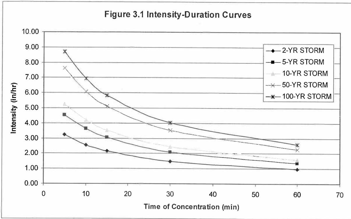
Factors for Preparation of Intensity-Duration Curves (Table RA-4 UDFCD June 2001)
