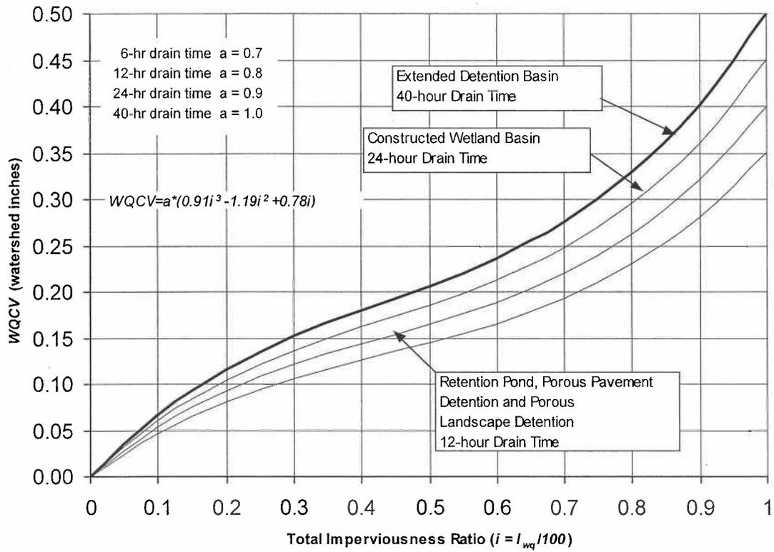
Figure EDB-2—Water Quality Capture Volume (WQCV), 80<sup>th</sup> Percentile Runoff Event
