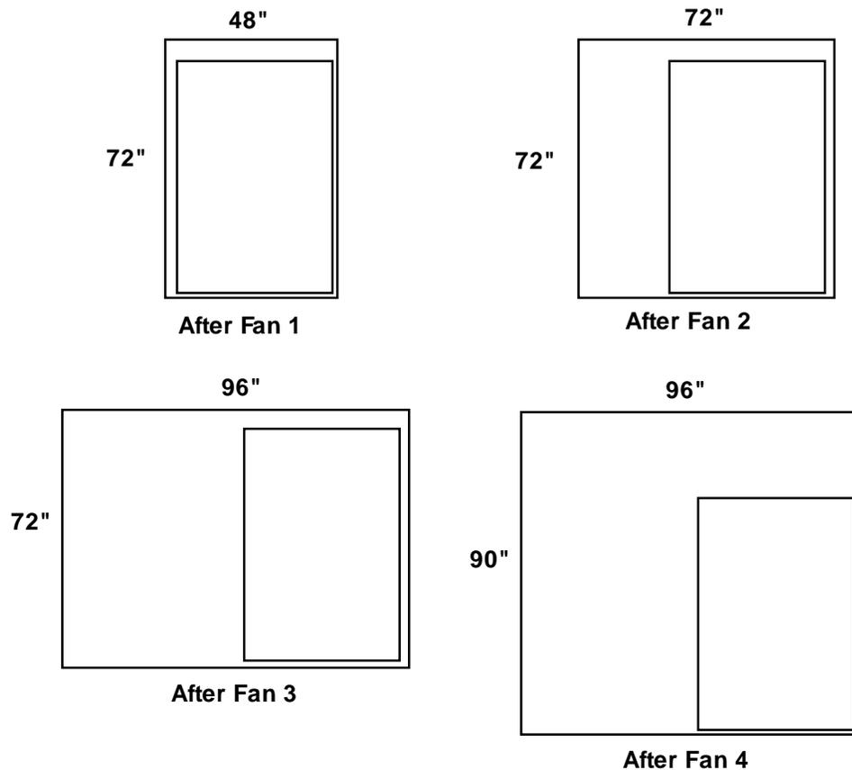
**Figure 3.** Changes in exhaust duct cross-section as fan exhaust outlets enter the discharge. Shaded areas show the approximate sizes and locations of the exhaust fan outlet ducts entering the main exhaust duct.
