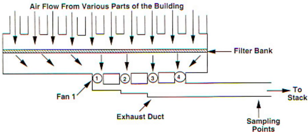
**Figure 2.** Schematic diagram of Building 771 exhaust system and location of effluent sampling points. This is a top view; it is not drawn to scale.
