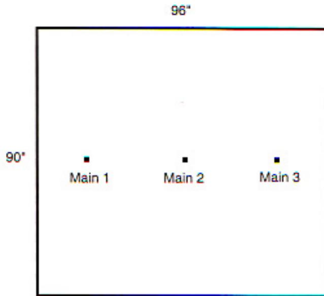
**Figure 1.** Locations of sampling points in a cross-section of the Building 771 exhaust duct after modification on 16 May 1963. Before that time samples had been collected only at the point labeled Main 2.
