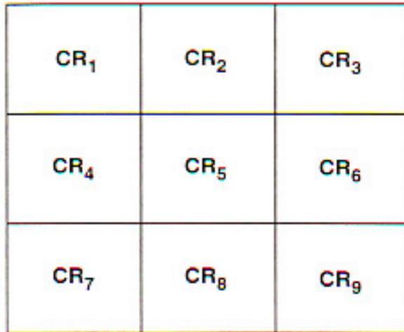
**Figure 4.** Illustration of the division of the exhaust duct into sectors. For the  $i^{\text{th}}$  sector, the concentration ratio ( $CR_i$ ) is the ratio of the concentration of plutonium in that sector to the measured concentration of the central sector.
