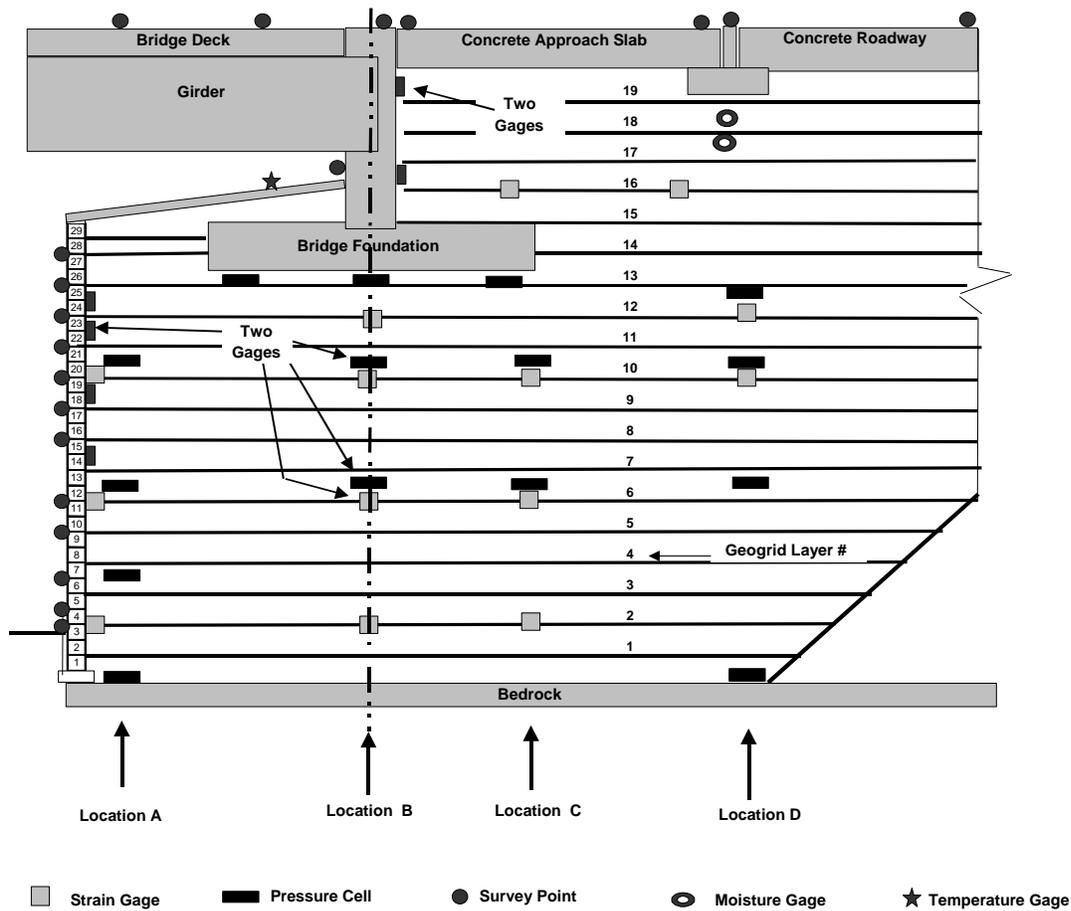
**Figure 12. Instrumentation layout at section 800 (phase II structure).**
