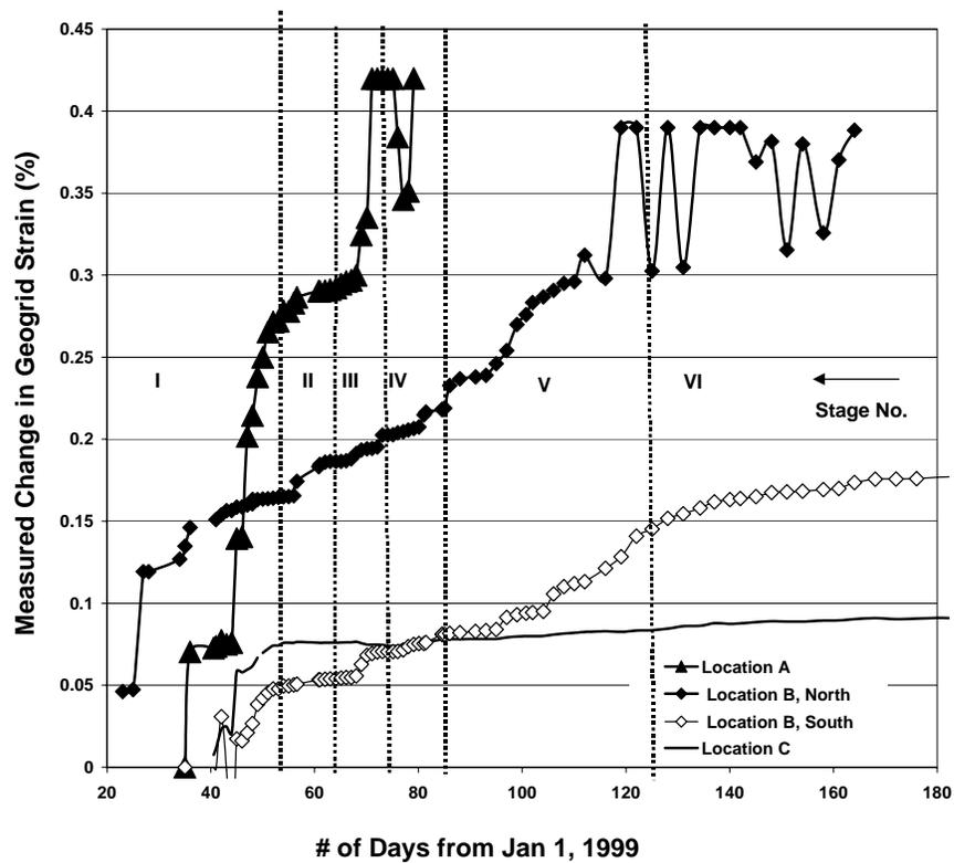
**Figure 14. Measured geogrid strains during all construction stages (measured on the 6<sup>th</sup> geogrid layer of section 800).**
