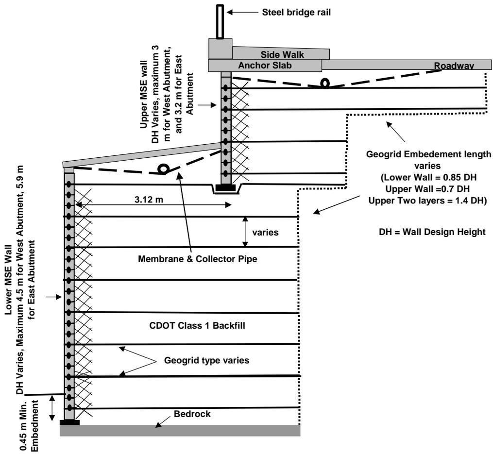
Figure 4. Typical cross-section along the upper and lower MSE walls (e.g., sections 300 and 900 in Figure 2).
