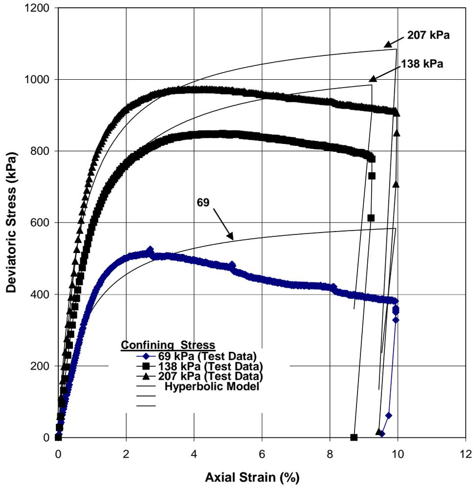
**Figure 6. Deviatoric stress-axial strain test results from large-size triaxial tests and predictions from hyperbolic model.**
