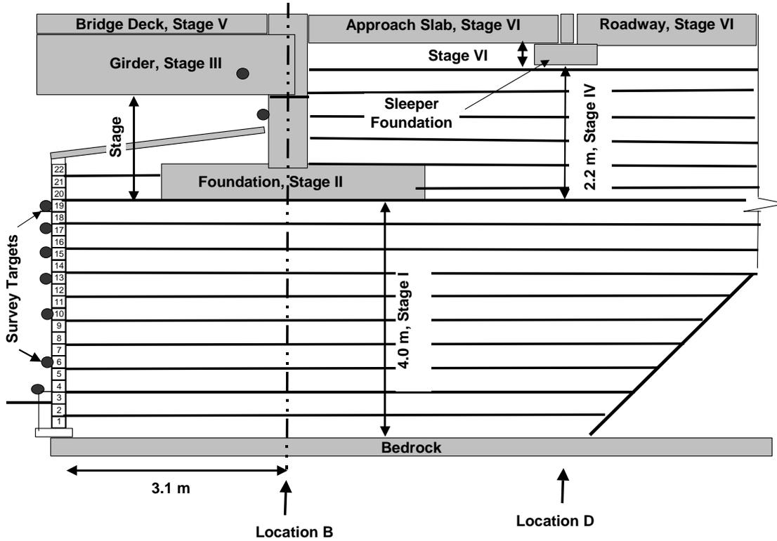
**Figure 8. Instrumented section 200 indicating construction stages.**
